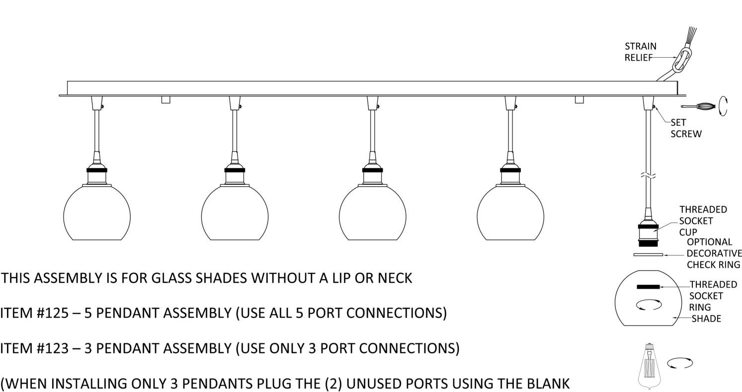
FEED THE CORDS THROUGH THE CANOPY PORTS AND TIGHTEN WITH THE TINY SET SCREWS IN THE PORTS, THEN PUT THE PLASTIC STRAIN RELIEFS ON THE CORDS DIRECTLY ABOVE THE CANOPY (TO KEEP THE CORDS FROM SLIPPING THROUGH THE PORTS). THEN SLIDE OPTIONAL DECEORATIVE CHECK RING AND SHADE ONTO THE THREADED SOCKET CUP AND SECURE USING THREADED SOCKET RING.
