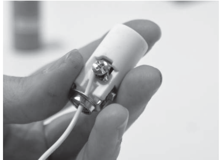
Do the same for the white wire and SILVER screw.
