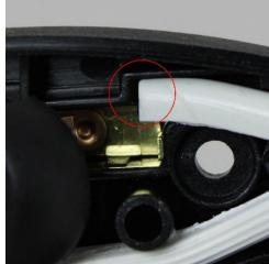
Step 4.) Press the cover down into the wire so that the notches push the wire into the piercing terminal and screw closed.
